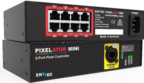
ENTTEC's PIXELATOR MINI is an 8-port Ethernet pixel controller. Using ENTTEC's PLINK protocol, each port provides data to ENTTEC's PLINK INJECTOR which can control up to 2 Universes each, making the PIXELATOR MINI powerful enough to control up to 8,192 channels (2,730 RGB Pixels) with perfect synchronization across all eight of its outputs.
