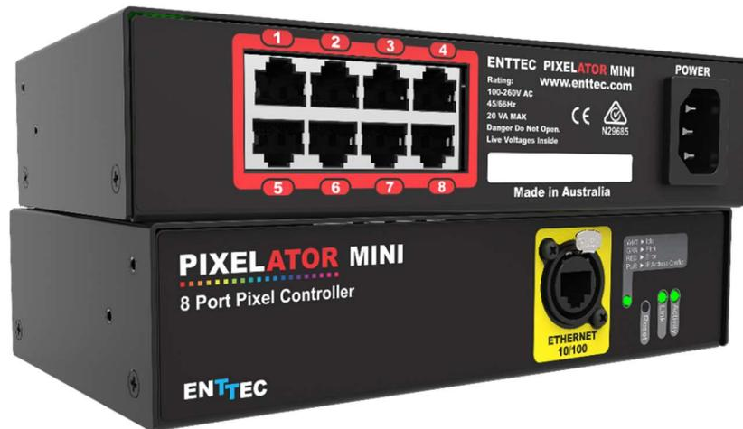
ENTTEC's PIXELATOR MINI is smaller 8-port half-width Ethernet pixel controller within the PIXELATOR family, perfectly suited to small and medium scale installations using ENTTEC's PLink protocol. Each PLink port provides data to ENTTEC's PLink Injectors which can control up to 2 Universes each, making the PIXELATOR MINI capable of controlling up to 8,192 channels (2,730 RGB Pixels) with perfect synchronization across all outputs.
